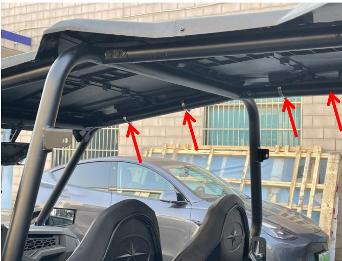
8. Press the circular plates with screws on the two U-shaped nut slots of the No. 4 roof frame.
