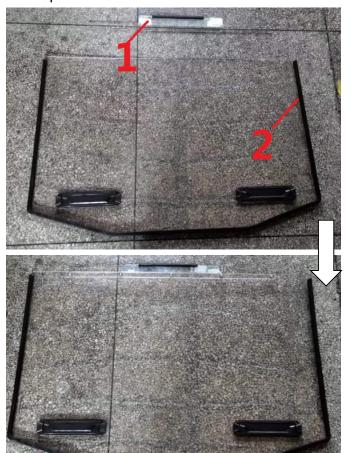
3. Remove the four screws on the front end of the plastic roof of the original vehicle, insert the lower end of the windshield into the gap of the front cover, and the upper end of the windshield against the front upper beam, as shown in the picture:
