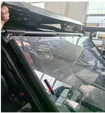
4. Tighten the four screws of plastic roof and fix the upper end of the front windshield on the front upper beam with two small ties, as shown in the picture:
