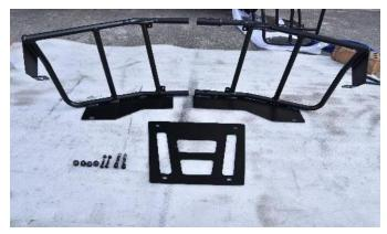
1. Assemble the separated cargo bed enclosure together with screws.Don't tighten the screws yet.As the picture shows:
