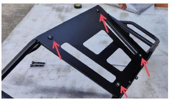
2. According to the marked position in the picture, remove the hardwares and tie downs from the cage for backup. As the picture shows:
