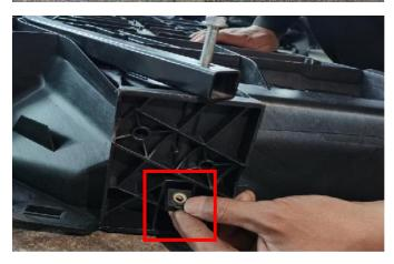
6. Install the new rear cargo box on the vehicle and secure it with the original screws of the vehicle.
