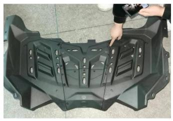
5. After removing the original rear cargo box from the vehicle, disassemble the skeleton and heat shield at the back as well as the movable nuts on both sides, and assemble it to the new rear cargo box in its original position.
