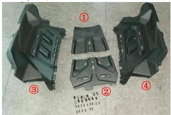
3. Snap the steel clips from the kit onto the fixing holes of attachment ②, and then use the screws to assemble attachments ① and ② together.
