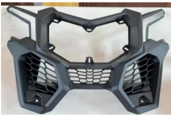
4. Remove the engine cover and front trim cover. As shown in the figure:
