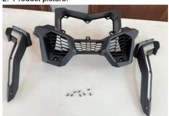
3. Remove the double-sided adhesive film on the daytime running lamp frame on both sides of the product, assemble the frame on the front fascia (distinguish the left and right sides). As shown in the figure:
