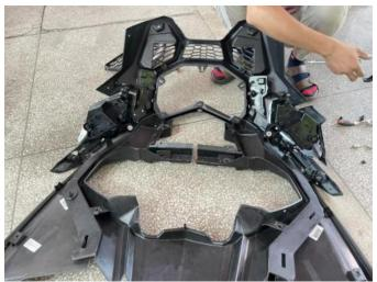
7. Refit the original grille and the brackets on both sides to the new front fascia. The reflectors on both sides of the original front bumper also need to be removed and fixed to the new front fascia. As shown in the figure:
