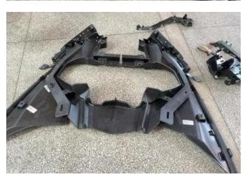
6. Clamp the steel clips just removed onto the new front fascia in the original position, then install the original daytime running lamps. After completing the previous steps, reassemble the front fascia onto the decorative cover plate, and then reinstall the original headlights. As shown in the figure:
