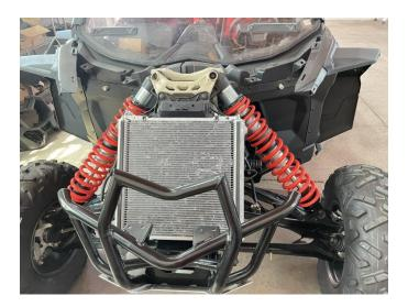
5. Remove the front fascia of the vehicle from the decorative cover plate, and the grille, daytime running lights and headlights of the vehicle also need to be dismantled. The removed screws and steel clips shall be kept for using later. As shown in the figure:
