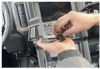
2. Use the matching screws to fix the mounting base on the original roof, and finally install the rearview mirror back on the mounting base. As the picture shows:
