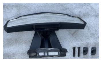
1. First, take out the two steel clips from the product accessories package, and insert them into the reserved holes of the original vehicle, and then remove the mirror from the mounting base. As the picture shows:
