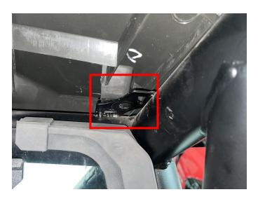
5. Move to the rear cargo box of the vehicle, prepare 6mm screw tap, drill out the screw holes reserved on the vehicle, and then use the screws and washers to fix the roof on the vehicle. As the picture shows:
