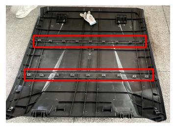
2. Fix with butt splint screws at the two ends of each splice. As the picture shows:
