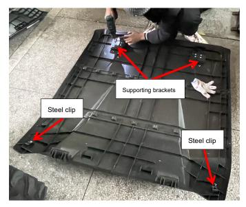
4. Place the assembled roof on the original vehicle, and clamp the front and rear fixing hooks on the original vehicle frame (the screw holes on the fixing hooks at the rear of the roof should be aligned with the screw holes reserved on the original vehicle frame for subsequent screw fixing), locate the steel clips, and use M6\*20 screws to fix them. As the picture shows:
