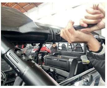
6. Finally, fix the supporting brackets on the roof top with self-tapping screws. As shown in the picture:
