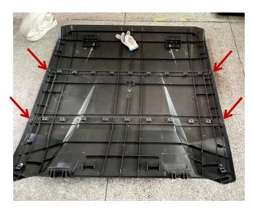
3. After assembling the matching supporting brackets, use M6\*16 self-tapping screws to fix the brackets on the roof, finally, place the steel clips in the place marked in the picture, as the picture shows:
