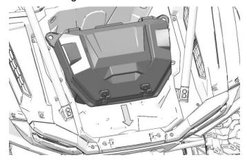
2. Install two Lock & Ride assemblies in two aligned mounting holes.
