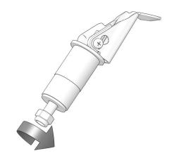
5. Make sure Lock & Ride assemblies are fully seated before closing top lever and securing storage box.
