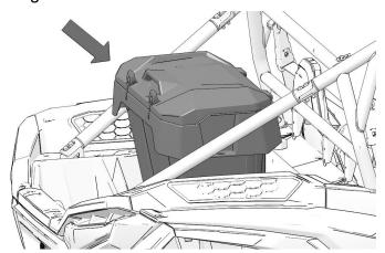
2. Move front of storage box to align Lock & Ride holes in storage box with those in cargo box.
