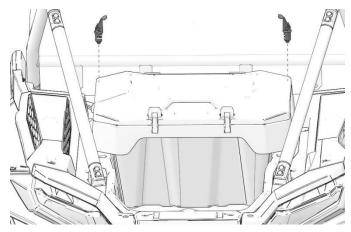
4. Lock & Ride assemblies may need adjustment. Tighten or loosen bottom nuts depending on fitment.
