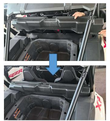
2. Install the rear windshield 1 on the plastic part 2, and lock the top three quick release devices:
