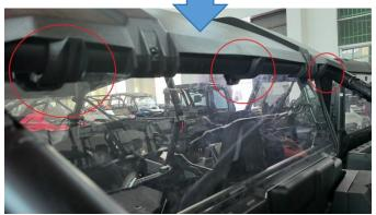
3. Connect the lower end of the rear windshield with the vehicle frame with three small straps, and the installation is completed.
