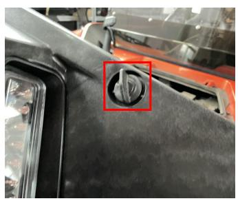
3. Take out the 2 extension cables in the accessories. One of which is connected to the vehicle's battery box, and the other is connected to the negative pole of the vehicle's electricity. After that, disconnect the rear half of the plug-in of the spotlight wiring harness of the hood. Then connect it with the other end of the two extension cables and do insulation protection well (one is black, and the other is red). As shown in the figure:
