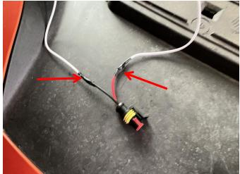
4. Connect the adapter plug-in to the spotlight wiring harness plug-in. Then put the hood scoop back onto the vehicle and fasten the hood clips. As the picture shows:
