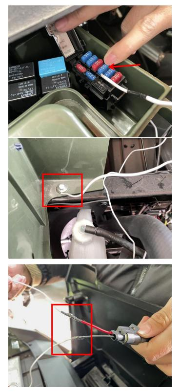
4. Connect the adapter plug-in to the spotlight wiring harness plug-in. Then put the hood scoop back onto the vehicle and fasten the hood clips. As the picture shows:
