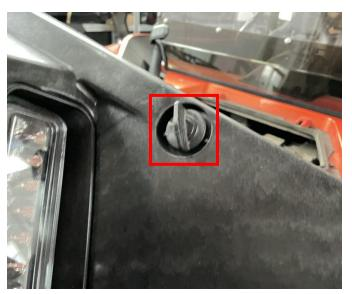
3. Put the hood back on the vehicle and fasten the hood clips. The installation is complete.
