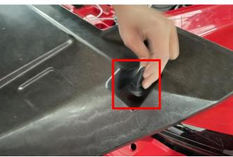
3. Put the cover back on the vehicle and fasten the hood clips.
