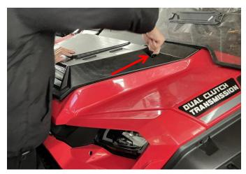
4. Connect the adapter plug-in to the spotlight wiring harness plug-in. Then put the cover back into the vehicle and fasten the hood clips. As the picture shows:
