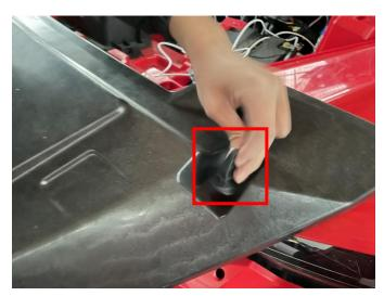
3. Take out the 2 extension cables in the accessories. One of which is connected to the vehicle's electrical box, and the other is connected to the negative pole of the vehicle's battery. After that, disconnect the rear half of the wiring harness plug-in on the spotlight of the cover. Then connect it with the other end of the two extension cables and do insulation protection well (one is black, and the other is red). As shown in the figure:
