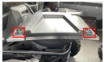
2. Install the new turbo hood on the vehicle, lock the switches. The installation finished. As the picture shows:
