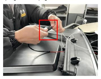
4. Install the new turbo hood on the vehicle, lock the switches. As the picture shows:
