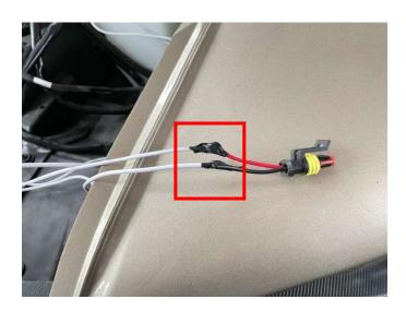
3. Connect the adapter harness plug-in to the spotlight harness plug-in.
