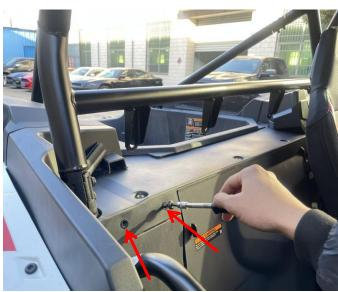
2. Thread the wiring harness of the speaker pod from the surface gap of the original vehicle to the bottom of the vehicle, and connect it with the plug-in reserved for the original vehicle, and finally use the original screws to fix the speaker pod. (The other side of the speaker pod can be installed in the same way). As the picture shows:
