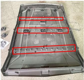
3. Clamp the matching steel clips to the fixed corners on both sides of the roof (stuck in the inside), and use M6\*16 screws to fix (each screw needs to be covered with a flat washer before use). As the picture shows:
