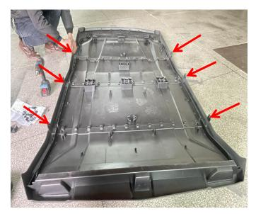
4. Use M6\*19 self-tapping screws to fix the brackets on the roof. As the picture shows:
