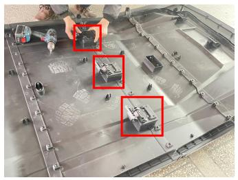
5. If the vehicle is a full door model, need to use tools to cut off the 6 fixed angles on both sides of the roof to avoid interference with the door frame (use M3\*12 self-tapping screws to fix the roof before cutting). As the picture shows:
