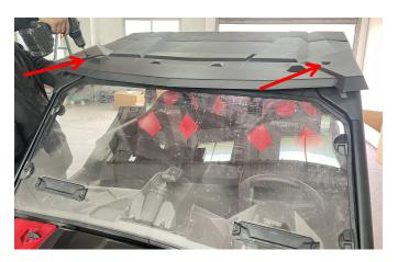
7. Clamp the roof brackets on the beam bar in the middle of the original vehicle, and use M6\*20 screws to fix it. As the picture shows:
