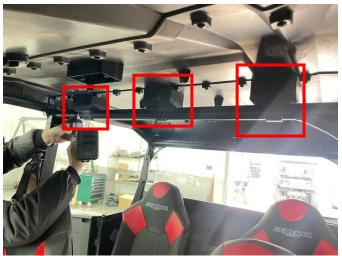
8. Attach the iron bracket supporting the roof to the middle section of the rear beam bar of the original vehicle, and then use M6\*20 screws to fix it. As the picture shows:
