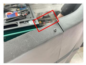
6. To place the assembled roof on the original vehicle, the limit hooks of the front end of the roof should be stuck into the notches of the original vehicle completely, and then install the steel clips on both sides of the top of the
