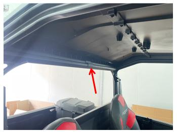
9. Finally, stick the fixed hooks on the side beam bar of the original vehicle, and then use the self-tapping screws to fix them (install total 8 fixed hooks, 4 on the left side, 4 on the right side). As the picture shows:
