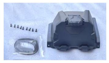
1.Place the navigation bracket on the center control console, then fix it with the self-tapping screws in the accessories package. Finally, take out the sponge strips in the accessories package. Stick the thick sponge strip to the lower part of the phone holder, and stick the thin sponge strip to the cover plate. As shown in the picture below:
