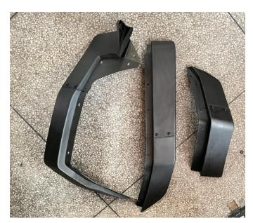
2. First, install the front fender flares: First, unscrew one screw from the original fender flares, and then place the assembled widened fender flares on the original fender flares (the fixing holes need to be aligned with the holes reserved in the original vehicle). Then, screw the original vehicle screws back in place and use the self tapping screws 5 \* 16 provided with the product to fix the fender flares. As the picture shows:
