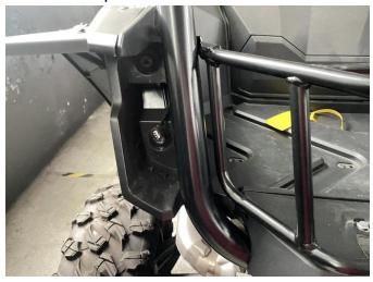
2. Connect the new tail light to the original vehicle wiring harness, and finally press the ball joint column on the rear shell of the new tail light firmly into the circular rubber hole of the original vehicle (you can add an appropriate amount of lubricating oil to the ball joint column for proper installation). (The tail light on the other side should be replaced and installed in the same way.) As shown in picture:
