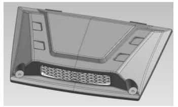
1. First, remove the original vehicle hood and move the hood clip onto the new hood. As the picture shows:
