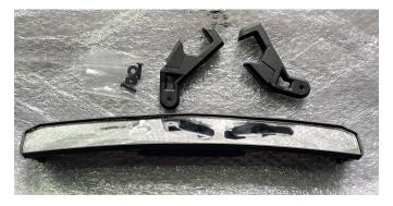
1. Use screws to secure the matching mounting bracket to both ends of the rearview mirror (a flat pad should be placed before and after the screws, and the screws do not need to be tightened during fixation). As the picture shows:
