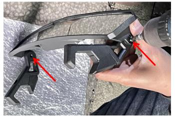
2. After loosening the screws on the mounting bracket of the rearview mirror, clip it onto the roof crossbeam (a non slip pad needs to be placed between the bracket and crossbeam), adjust the left and right distances, and then tighten the screws on the bracket. As the picture shows:
