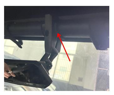
3. After adjusting the rearview mirror to the appropriate angle, tighten the screws at both ends.As the picture shows:
