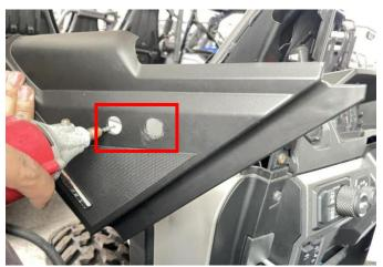
3. Fix the base support of the mirror to the A-pillar with M6\*20 screws, reinstall the A-pillar guard plate and secure the buckle. Finally fix the mirror to the base support with M8\*45 screws. (The other side mirror is installed in the same way as above). As the picture shows:
