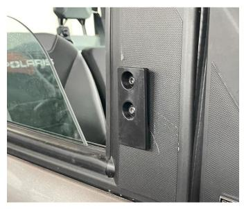
4. Finally, clamp the corresponding side of the mirror down on the base, and then use M4\*12 self-tapping screws to fix it (the other side of the mirror is installed in the same way as above). As the picture shows:
