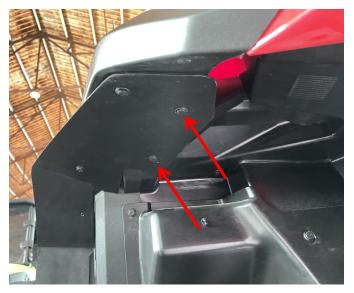
3. Drill holes at the 2 positioning holes on the top of the mud flaps with an 8mm drill bit, and fix them with buckles, as shown in the figure:
