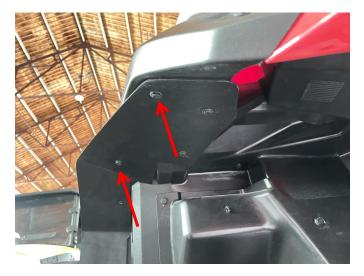
4. The remaining positioning holes on the mud flaps can be fixed by using the self-tapping screws and the flat pad in the kit. (Install the other side in the same way as above). As the picture shows:
