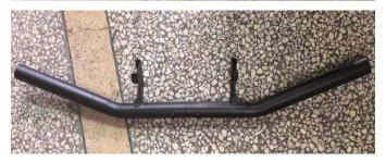
3. Remove 4pcs screws and 4pcs nuts from the back of the vehicle and save them for later use. The rear bar is then secured to the frame with 4pcs removed screws and 4pcs nuts. As shown in the picture:
