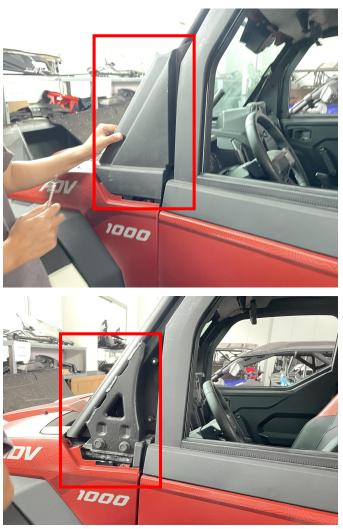
3. Install the new guard plate with side mirror on the A-pillar in the same way, and fix it with the matching screws and snap fasteners. (The other side of the mirror can be replaced and installed in the same way as above). As shown in the picture:
