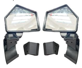
1. First distinguish the left and right sides of the rear view mirrors, and then find the right height on the original A-pillar, clamp the bracket of the mirror on the pillar, and push backwards with your palms at the same time, to make the claw be stuck more firmly on the pillar. As shown in the picture:
