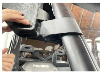
2. Use the matching iron bracket, hook one side on the pillar, and fix the other side on the mirror with screws, to make it hold the mirror better. (The other side of the side mirror can be installed in the same way as above). As shown in the picture:
