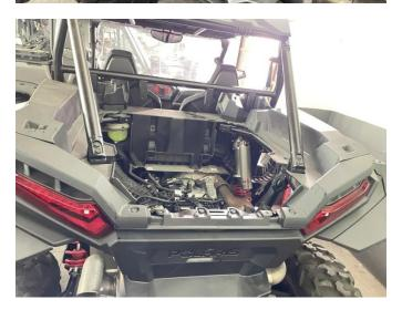
3. Use the matching M5 screws and flat washer nuts to fix the installation locks on the original rear cargo box, as shown in the picture:
