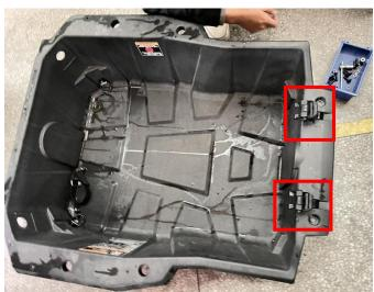
4. Place the cover on the rear cargo box, prepare a 6mm drill bit, drill holes according to the positions of the fixing holes on the cover, and secure the cover by M6\*20 screws and flat washer nuts. As the picture shows:
