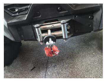
3. Fix the upper end of the front bumper to the frame with two M12 \* 30 external hex screws. As shown in picture:
