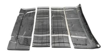
1. First, stick the sponge strip with adhesive in the accessory package to the junction edge of the middle two roof panels (on the side of the roof surface), and then use M6 \* 16 self tapping screws to assemble the four roof panels into a whole. As the picture shows:
