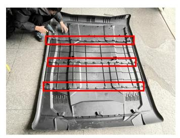
2. Use M5 \* 16 self tapping screws to secure the two mounting iron brackets to the roof. As the picture shows:
