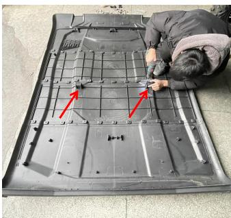
3. Prepare a 6mm drill bit and secure it using M6 \* 16 screws and matching nuts according to the positioning holes on the roof (a flat pad is required on each screw). As the picture shows:
