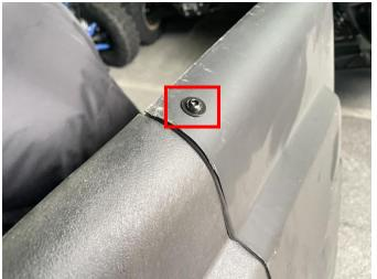
4. Install the assembled roof onto the original vehicle, place the pressure plate with nuts in the groove at the front of the roof, and fix it from below using M6 \* 16 screws. As the picture shows:
