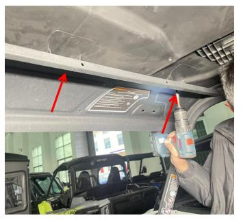
5. Thread the matching steel hoop through the installation bracket on the roof, wrap it around the crossbeam in the middle of the original vehicle, and then tighten the screws on the steel hoop. As the picture shows:
