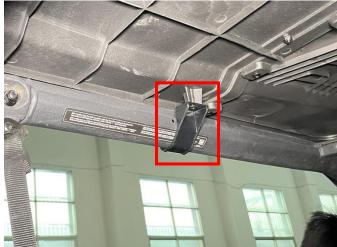
7. Finally, use stainless steel hex screws to secure the iron pressure plate to both sides of the rear of the roof. As the picture shows:
