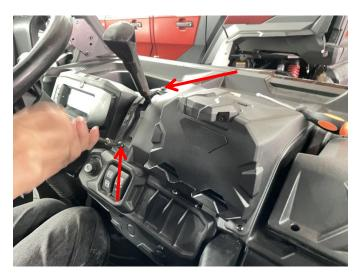
2. Use the self tapping screws in the accessory package and fix them in sequence according to the positioning holes around the tablet holder. As the picture shows:
