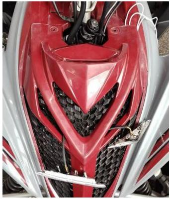
3. Clamp the lights in the corresponding position on the front cover. As the picture shows:
