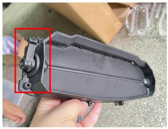
5. Use M3\*20 self-tapping screws to fix the adjusting wrench on the top of the air vent port.
