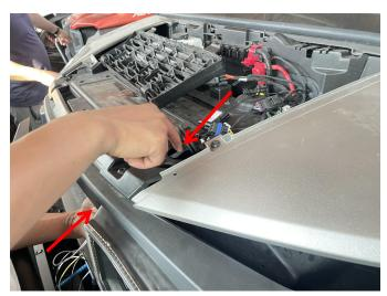
4. Remove the grille. Connect the matching harness to the copper pin on the light, and pass the excess wiring harness through the gap in the front, and then through the cable hole on the top of the vehicle. As the picture shows:
