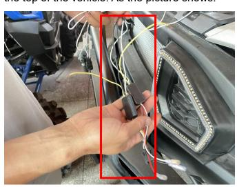
5. Connect the pulled wiring harness to the corresponding plug-in on the matched conversion harness. Disconnect the wiring harness plug-in of the headlight, and then re-connect the conversion harness with the headlight and the vehicle wiring harness plug-in. After completion, turn on the switch to check whether the light is on normally, and after confirming that it is correct, the grille and the hood cover can be installed back. As the picture shows:
