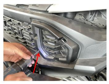
3. Pass the light wiring harness through the newly expanded hole, then press hard to clamp the light on the corresponding slots of the fascia. (The other side of the light is installed in the same way). As the picture shows:
