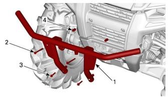
5. Secure bumper with M8 Elastic hex. nuts and tighten them.
