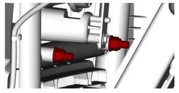
6. Reinstall radiator air deflectors with previously removed plastic rivet. The installation is complete.
