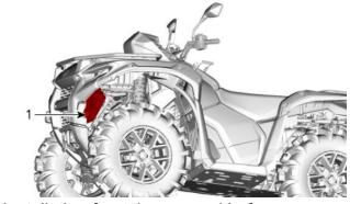
4. Install the front bumper with four screws. Use two M8x95 hex screws with two spacers for the upper part and two M8x45 hex screws for the lower part.
