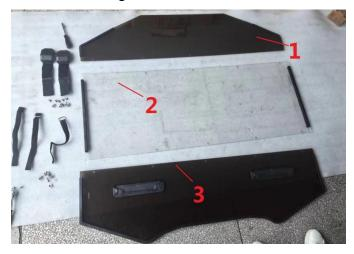
3. Assemble the windshield with 10 M6\*20 screws, 10 M6 lock nuts and 10 M6 spacers.
