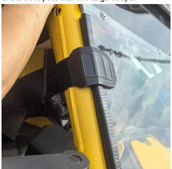
7. Fix the top of the front windshield on the frame with two small straps and complete the installation.
