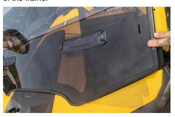
5. Open the plastic panels on the left and right sides and secure the lower end of the windshield to the front post with two small straps.
