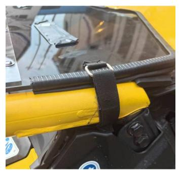
6. Secure the middle position of the windshield to the front post with two large straps.
