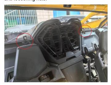
6. Secure the top end of the rear windshield to the rear frame with two straps, installation complete.
