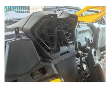
4. Secure the rear window to the rear post first with two straps.
