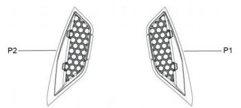
2. Install LH grille insert [P1] in place starting by the two outer tabs and then the inner tab.
