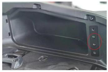
3. Snap the front end of the baffle into the two slots and tighten the back end with 2 quick release screws (Install the other side in the same way).
