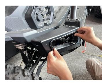
3. Distinguish the left and right sides of the lights, align the mounting tabs position, and then fix the light on the front bumper with screws (the other side is installed in the same way). As the pictures show:
