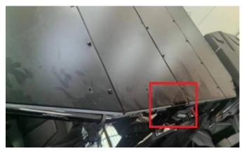
5. Fix the roof to the frame with 12pcs brackets (Part 7),12pcs hex screws of M6\*30, and 12pcs nuts. As shown in the figure:
