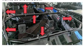
4. Place the roof on the top of the frame, and the notch position is aligned with the frame position, as shown in the figure:
