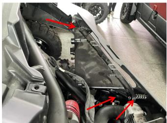
2. Disconnect the harness plug-ins of the original headlight, remove the original headlight and replace it with a new headlight, and use the original screws to fix it, and then connect the original wiring harness with the new headlight (the other side of the headlight is replaced and installed in the same way), and then finally install the removed parts back in place. As shown in the picture:
