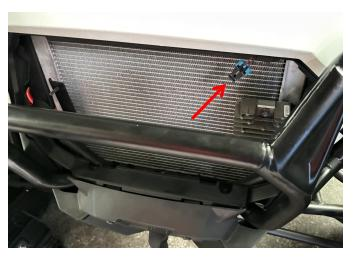
2. Disconnect the wiring harness plug-ins of the spotlight on new mesh grill first, and connect the wiring harness to the extension wiring harness of the original vehicle by breaking the outer skin of the wire (connect the black wire to the black wire, and connect the red wire to the red wire), the wire junction must be insulated, and then reconnect the wiring harness plug-ins. Finally fix the mesh grill. As the picture shows:
