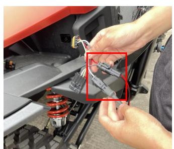
3. Disconnect the wiring harness plug-in of the original headlight, and connect the wiring harness of the original headlight with the plug-in on the conversion cord, and finally
