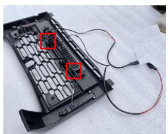
2. Pull the connected extension wire and spotlight harness through the gap of the vehicle to the headlight position on the driver side, and then connect with the matching conversion cord. As the picture shows:
