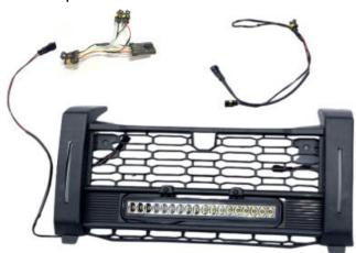
1. First, remove the original front mesh grill, and move the fixed locks of the original mesh grill to the new mesh grill, and connect the matching extension wire with the wiring harness plug-in of the day running lights. As the picture shows:
