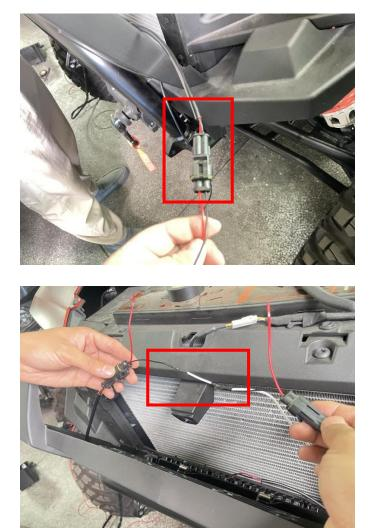
2. Connect the other end of the extension wire to the negative terminal of the original vehicle battery. As the picture shows:
