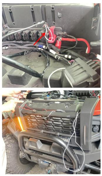
3. Pull the wiring harness of the center spotlight to the headlight on the driver side through the gap of the vehicle, and disconnect the wiring harness of the original vehicle headlight, use the conversion wire matching with the center spotlight to re-connect the original vehicle headlight and the vehicle wiring harness, and finally connect the plug-in reserved on the conversion wire (the plug-in of the black and white wire) to the spotlight wiring harness. As the picture shows:
