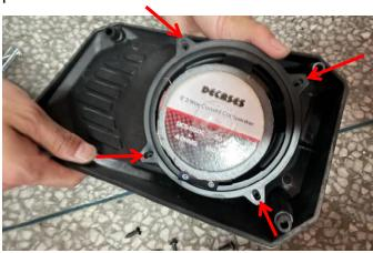
2. Prepare a 3mm drill bit and drill holes according to the reserved anchor points where the speaker is installed on the original vehicle. Then match the bracket to the fixing holes, secure it using M4\*30 self-tapping screws (the other side is installed in the same way). As the picture shows:
