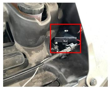
4. After reconnecting the previously disconnected middle grille light harness, the double-sided adhesive film on the surface of the drive box can be peeled off, and the drive box can be affixed to the original vehicle gap. As shown in picture:
