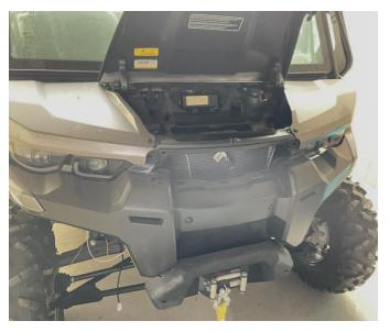
3. Disconnect the controller harness on the grille light, then prepare 2 extension wires. Connect the 2 extension wires to the just disconnected half of the harness, then pull the positive extension wire through the vehicle gap to the ACC electrical box and connect it to the electrical box. Pull the negative extension wire to the original headlight and connect it to the black wire on the headlight harness. The interface needs to be insulated and protected. As shown in picture:
